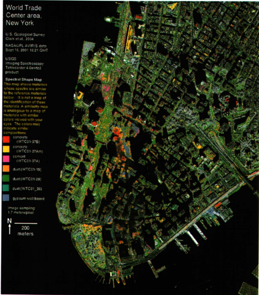
Plate 4.4. Map showing the WTC dust and debris plume as detected by AVIRIS indicating an asymmetry in the dust and debris distribution, with more iron bearing materials to the south by southeast.
